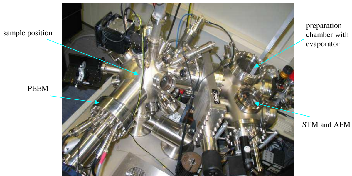
FIGURE 3-13: PEEM UHV-tool at TU Kaiserslautern [113].
